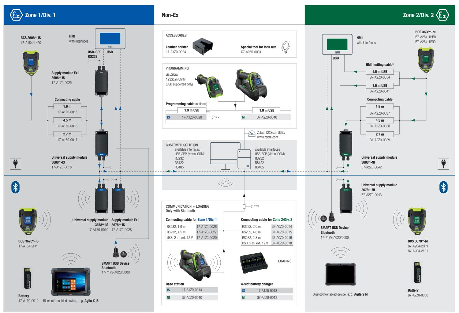
—C Power supply options: DC 24 V, AC 110/120 V, AC 230 V ---- Customer specific connecting cable — BARTEC specific cable
