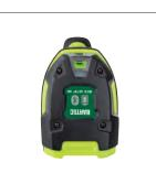
The Bluetooth version is ideal for mobile applications used to collect data from 1D barcodes, 2D barcodes, postcodes and OCR in a potentially explosive atmosphere (Transfer of photos to the host PC is only possible via the base station). The rugged version offers all highly developed ergonomic and functional features required in industrial applications. For the Bluetooth version there are several possibilities to transfer the data via Bluetooth "Single Point-to-Point".
